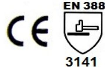
Tested in accordance with the European directive for PPE (89/686/EEC) for simple design, and is compliant with EN 420, EN 388.
